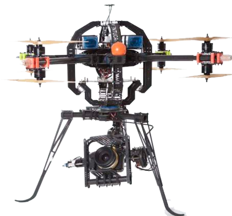
Hammer X8 MTOW 16 kg max speed 80 km/h
